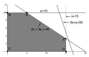
To find the maximum value of 6x + 8y and a point (x, y) in the feasible set at which it is achieved, we need only calculate the co-ordinates of the points A, B, C, D and E and compare the value of 6x + 8y at each.
